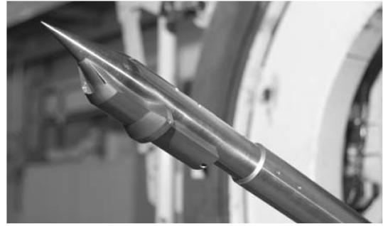
Fig. 2 Assembled 90-deg intake model at \alpha = 30 deg.
